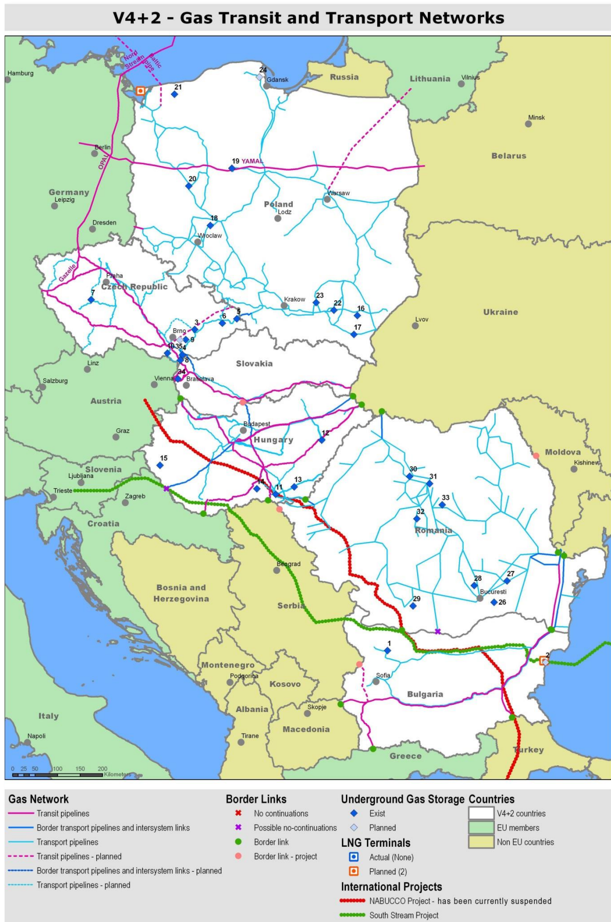
Figure 7: Gas transmission network
